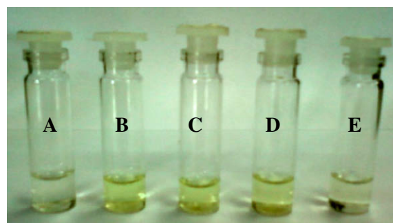
Figure 4. Color change of receptor 1 (A) upon addition of 1 equiv of different tetrabutylammonium salts of (B) acetate, (C) pivalate, (D) phenyl acetate, and (E) fluoride in acetonitrile.
